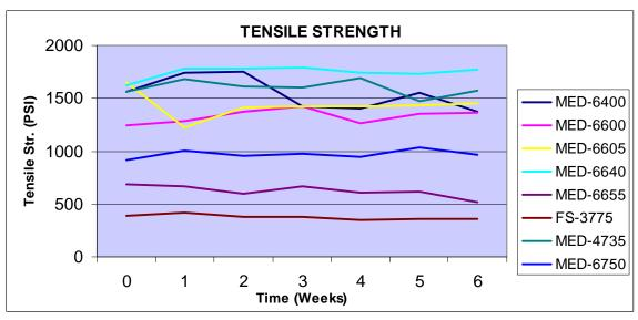
Figure 2: Tensile Strength results over 6 weeks.
